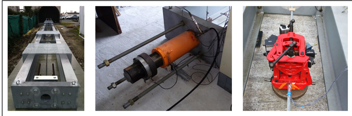
Figure 14. Test bench. From left to right: bench structure, jack and load cell, and additional mass to create a point load.
