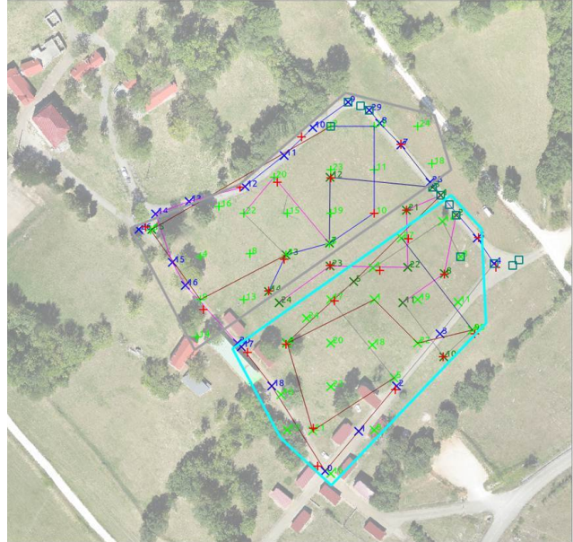
Fig. 8 Screenshot of the mission preparation software. Each red cross is a point to observe. The allowed positions for the AAV are in light green (encompassed in two safety zones in cyan and gray). For the two types of AGV, there are in blue and dark green. In addition, the patrols are drawn between allowed positions. The green squares represent the starting points of the robots.
