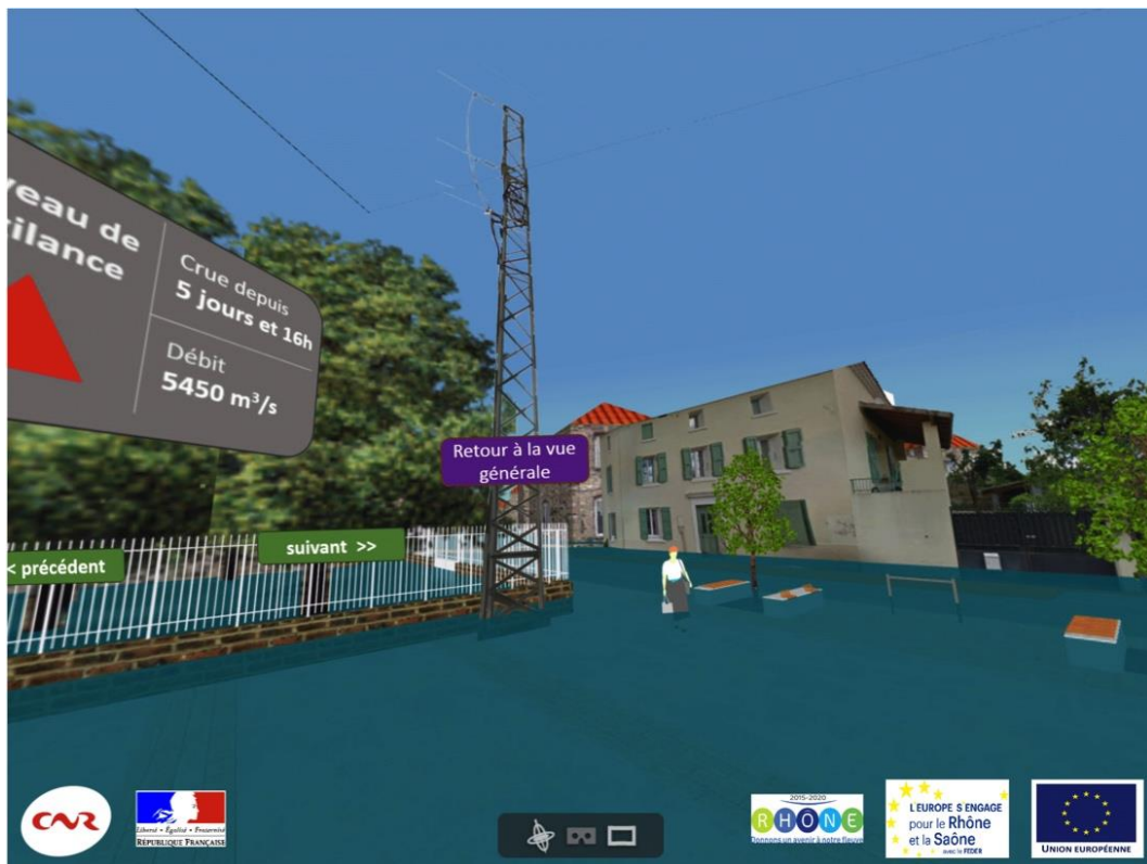
Figure 5. Example of the 360° images produced for immersive visualization (with a smartphone inserted into a virtual reality (VR) headset). Purple and green panels can be used to navigate between different moments in time (during the simulated flood). Grey panel gives information about water flows ( m^3 per second), point in time (number of days since the beginning of the flood), and the corresponding level of vigilance (here red).
