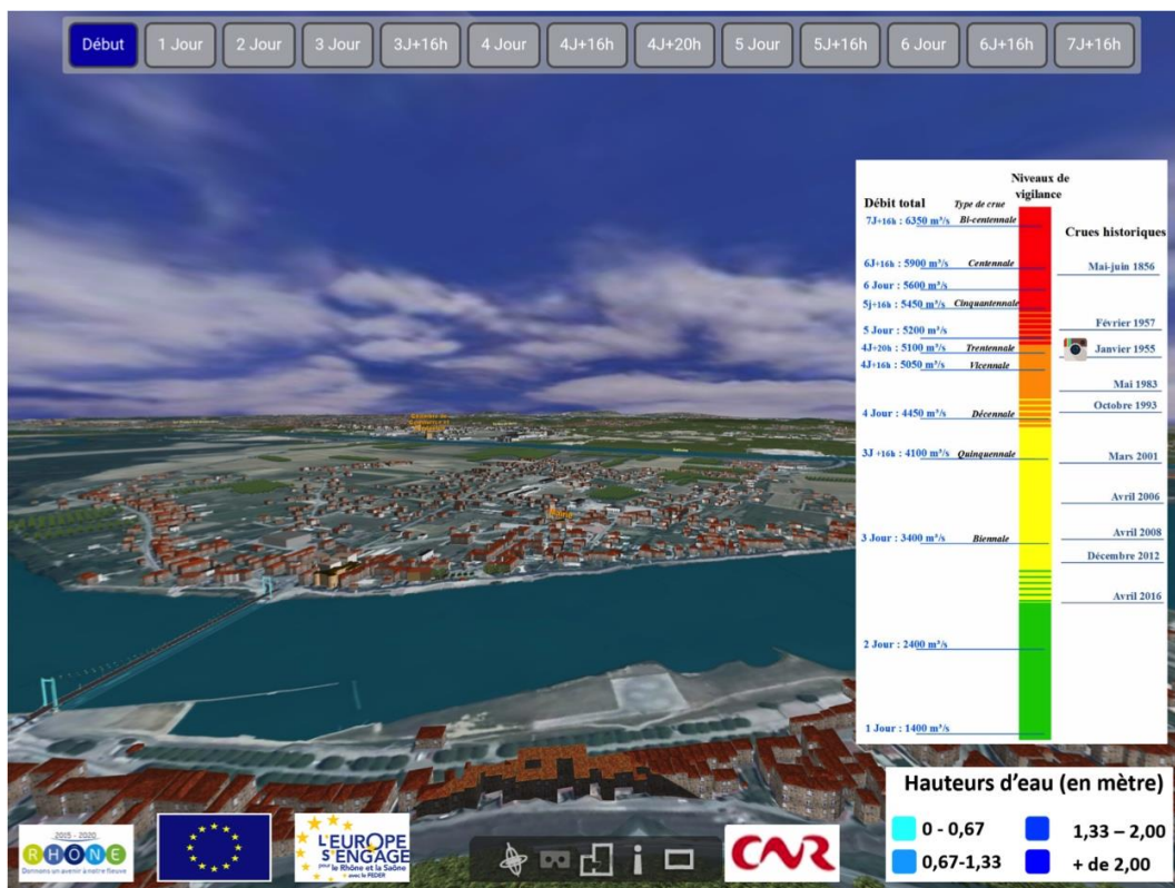
Figure 4. Interface proposed to the public on tablets for the visualization of the simulated flood from a chosen point of view. At the top is a temporal navigation panel to choose a point in the timeline of the simulated flood. On the right is a panel that can be hidden or displayed and that provide a link between water flow (m 3 per second) and historical floods that have occurred on the territory. It also enables the user to access historical pictures for some historical floods. At the bottom is a spatial navigation panel to go to the left or right, look up or down and zoom in or out. The information tool gives more details on how the flood was simulated.
