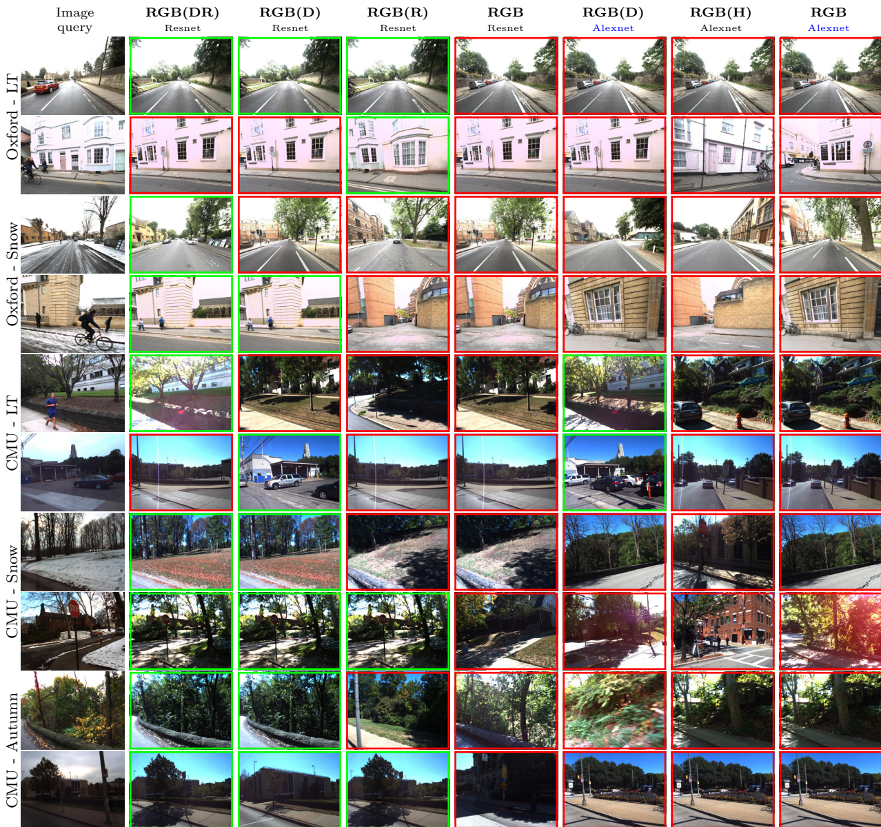
Fig. 7 Visual inspection of selected examples: we show top-1 retrieved candidate after the nearest neighbor search for the different descriptor. Red box indicates a wrong match and green box a proper one ( i.e. retrieved image lies in 25m radius from the query ground truth position). RGB([D/R/DR]) are our descriptor trained with, respectively, depth, reflectance, depth and reflectance auxiliary modality.
