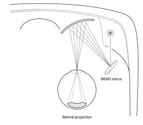
Figure 3: QD-Laser VISIRIUM® technology using a MEMS mirror and a free-form reflecting mirror <sup>2</sup>.
