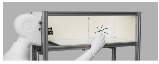
Figure 1: Overview of the experimental setup. The participant had his head on a chinrest and was able to see virtual elements with an OST device or a RPD. He was asked to point a target (virtual or real) with his finger (wearing a tracked ring). The frame was covered by white panels to prevent the participant from seeing his hand. (Here, one panel is transparent for illustration purpose).
