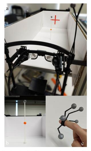
Figure 4: (a) Overview of the experimental system, here with the RPD. The red cross is used only for the calibration and removed during the experiment itself. (b) The real pole with the orange sphere used as target with the reflective tracking marker on the top. (c) The 3D printed ring used to support 5 reflective tracking markers and provide the position of the fingertip.
