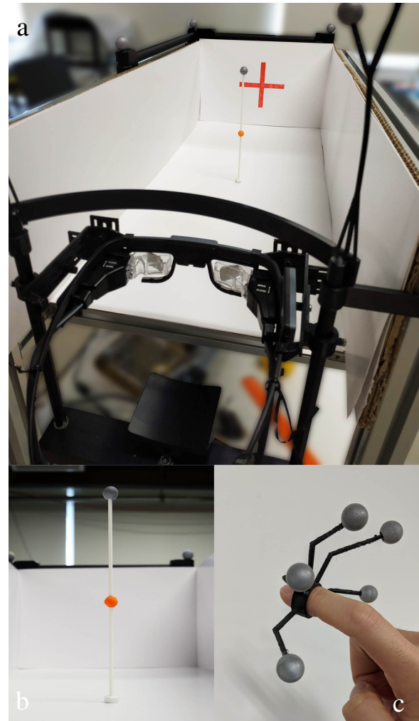
Figure 4: (a) Overview of the experimental system, here with the RPD. The red cross is used only for the calibration and removed during the experiment itself. (b) The real pole with the orange sphere used as target with the reflective tracking marker on the top. (c) The 3D printed ring used to support 5 reflective tracking markers and provide the position of the fingertip.
