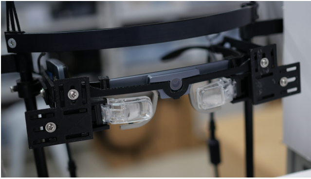
Figure 6: Close-up of the custom binocular headset with its two RPD modules mounted on an eye tracking device.
