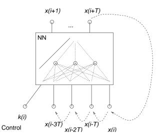
Fig. 1: Input/Output structure of the neural model.
