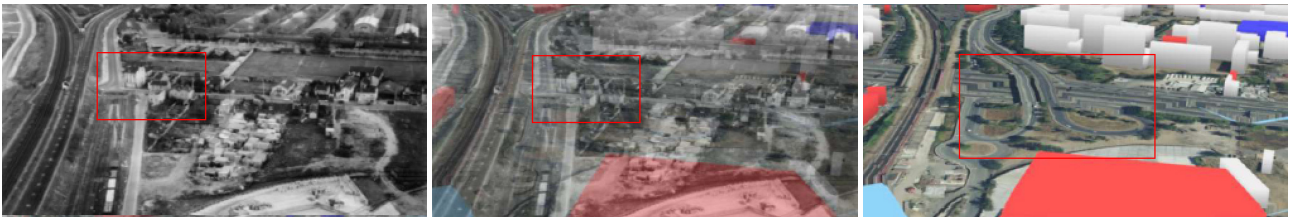
Figure 12. Interaction between a photograph (left) and the 3D scene (right) through transparency (middle). Infrastructure evolution and (dis)appearance of landmarks (hotel/restaurant vs highway interchange) are highlighted (©AD92, period 1960-1961).
