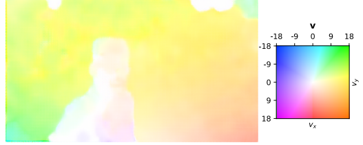
(d) Optical flow \mathbf{v} . Displacements are in pixels.
