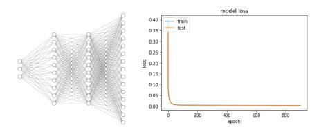
Figure 3: The Neural Network has 3 inputs, two hidden layers each with 50 neurons (10 shown here) and separated by batch-normalisation and an output layer with M output (M=15 shown here). Right: typical convergence curve of the loss function during the training phase.
