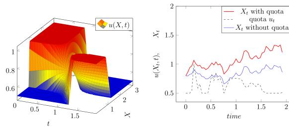
Figure 20: Optimal biomass and quota function Figure 19: Solution of the dynamic programming computed by Optimal Control and compared with the solution with  $u = u_M$  when  $X_0 = 0.8$ .
