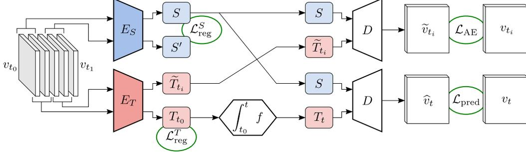
Figure 1: Computational graph of the proposed model.  $E_S$  and  $E_T$  take contiguous observations as input; time invariance is enforced on  $S$ ; the evolution of  $T_t$  is modeled with an ODE and is constrained to coincide with  $E_T$ ;  $T_{t_0}$  is regularized; forecasting equates to decoding from  $S$  and  $T_t$ .
