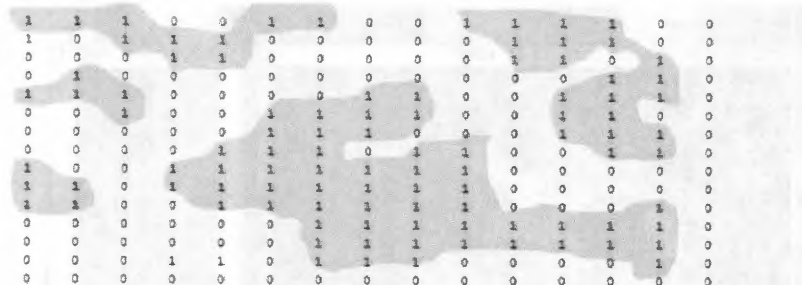
Figure 7.7 Illustration of 2D connected particles in a 2D mask; in 3D the same principle holds but each voxel has 26 neighbors instead of 8.
