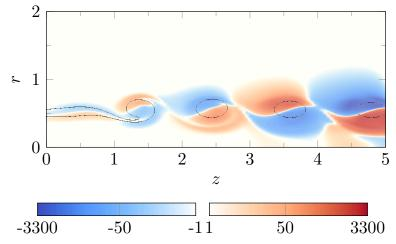
Figure 11:  $\mathcal{L}_2$  norm optimal vorticity response  $\omega'_{2,\theta,opt}$  snapshot Re = 2000 and St = 0.50 at a zero phase. A level-4 contours of base flow vorticity has been added to understand the response pattern. A truncated and sign-sensitive logarithmic scale has been used.
