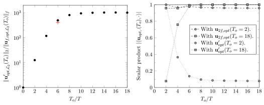
Evolution of the optimal gain. Black (a) circles denote values obtained for the standard cases without phase shift between harmonic and subharmonic forcing, red crosses represent the gain obtained with the phase shifts discussed in respect to the relevant  $\mathcal{L}_2$  norm. §**3.4.4**.
