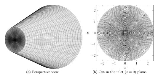
Figure 18: Mesh used for 3D nonlinear computation.
