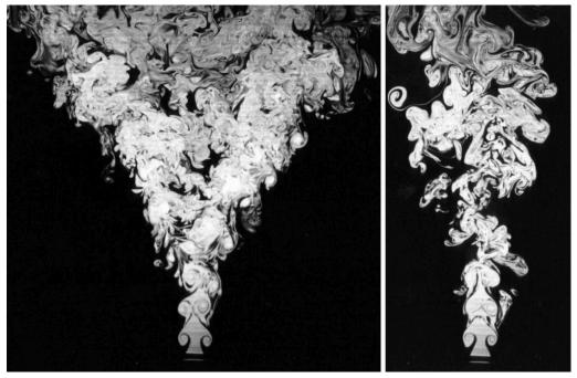
Figure 1: Bifurcating (left) and bisecting (right) plane views of a bifurcating jet at Re = 4300 with  $R_f = 2$ . From Lee & Reynolds (1985).
