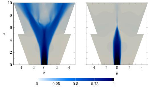
Figure 20: Mean axial velocity cut in the bifurcating (y = 0, left) and bisecting (x = 0, right) planes for the Re = 2000, St = 0.5 case optimally forced with a 1% amplitude. The sponge layers are not displayed.
