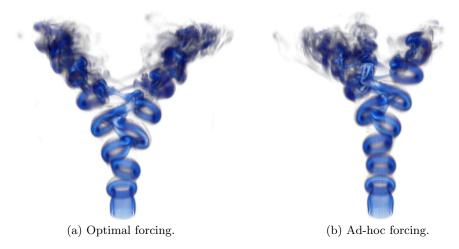
Figure 19: 3D vorticity magnitude snapshots of the nonlinearly forced bifurcating jet for Re = 2000 and St = 0.5. On the left, the jet is forced optimally, whereas on the right, simple ad-hoc forcing is applied.
