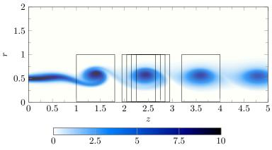
Figure 7: Vorticity cut of the Re = 2000, St = 0.50 base unpaired flow, with vortex domains represented for the first three vortices. For the second vortex, four  $\delta_z$  sizes are sketched (0.4, 0.6, 0.8, 1.0), whereas for the first and third ones, only the  $\delta_z = 0.8$  box is represented.
