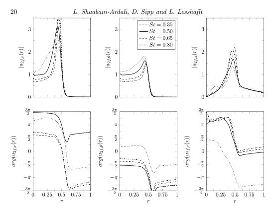
Figure 13: Evolution of the  $\mathcal{L}_2$  norm optimal forcing modulus and phase for four different Strouhal numbers.  $|\mathbf{u}_{2\mathbf{f}}(r)|$  and  $arg(\mathbf{u}_{2\mathbf{f}}(r))$  are defined in equation (3.2).
