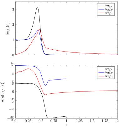
Figure 10:  $\mathcal{L}_2$  norm optimal forcing modulus and phase for Re = 2000 and St = 0.50. The phase was unwrapped to remain continuous in r.  $|\mathbf{u}_{2\mathbf{f}}(r)|$  and  $arg(\mathbf{u}_{2\mathbf{f}}(r))$  are defined in equation (3.2).
