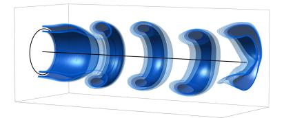
Figure 12: Snapshot of the superposition of the base flow and of the  $\mathcal{L}_2$ -norm optimal response with a finite amplitude at Re = 2000 and St = 0.5.
