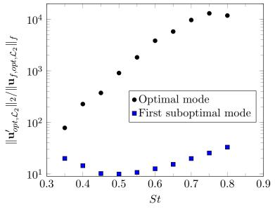
Figure 14: Evolution of the long-term  $(T_o \rightarrow \infty)$  optimal and first suboptimal gains for the  $\mathcal{L}_2$  norm optimisation as a function of Strouhal number.
