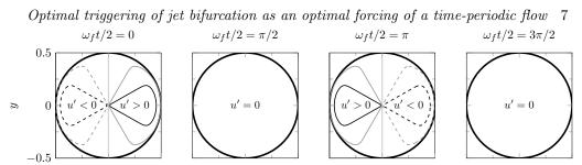
(a)  $u'(r, \theta, z = 0, t) = U_0(r) \cos(\theta) \cos(\omega_f t/2)$ . In this case, a constant vertical symmetry plane is observed.
