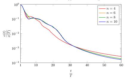
Figure 6: For different mesh resolutions (polynomial order n of individual spectral elements), the norm e(t) of the residual difference between the flow velocity at time t and time  $t - T_f$  is traced as a function of t. These are the stabilised computations (with source term 2.4) performed to find the periodic base flow at Re = 2000 and St = 0.6. The converged setting n = 8 is used in the following.
