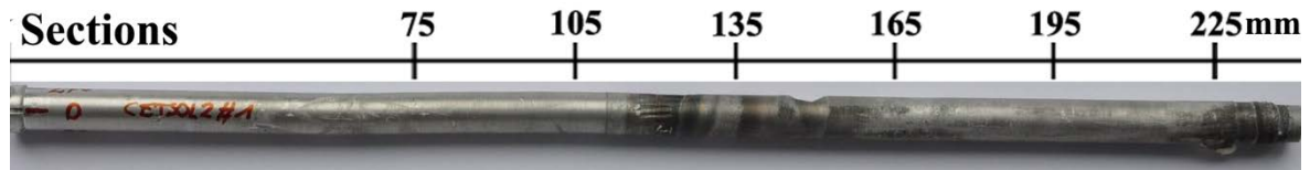
4 5 Fig.3. Optical image of the processed sample B2F1 with the identification of the cross-section 6 positions.
