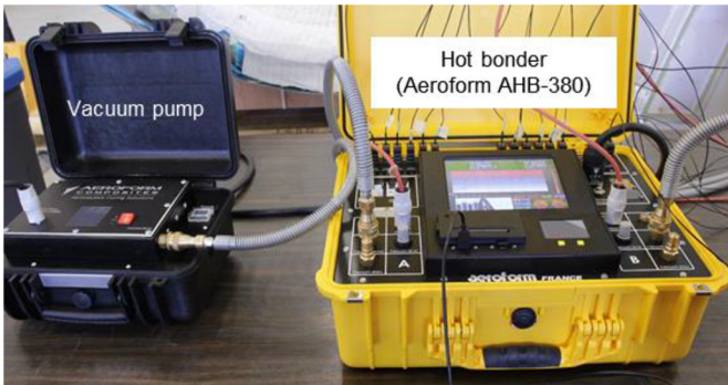
Fig. 13. Portable hot bonder Aeroform AHB-380 (right) and the portable vacuum pump (left).
