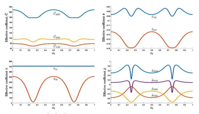
**Fig. 3.** Effective coefficients components  $\hat{C}_{3333}$ ,  $\hat{C}_{2323}$ ,  $\hat{c}_{1133}$  (stiffness),  $\hat{e}_{123}$ ,  $\hat{e}_{312}$  (piezoelectric),  $\hat{\kappa}_{11}$ ,  $\hat{\kappa}_{33}$  (relative effective permittivity) and  $\hat{\mu}_{3333}$ ,  $\hat{\mu}_{3131}$ ,  $\hat{\mu}_{1231}$  (flexoelectric).
