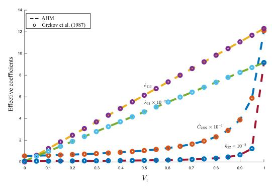
Fig. 2. Comparison of the effective coefficients  $C_{2222}$ ,  $e_{113}$ ,  $\kappa_{11}$  and  $\kappa_{22}$  obtained using the formulas (45), (48),(49) and the model described in [22].
