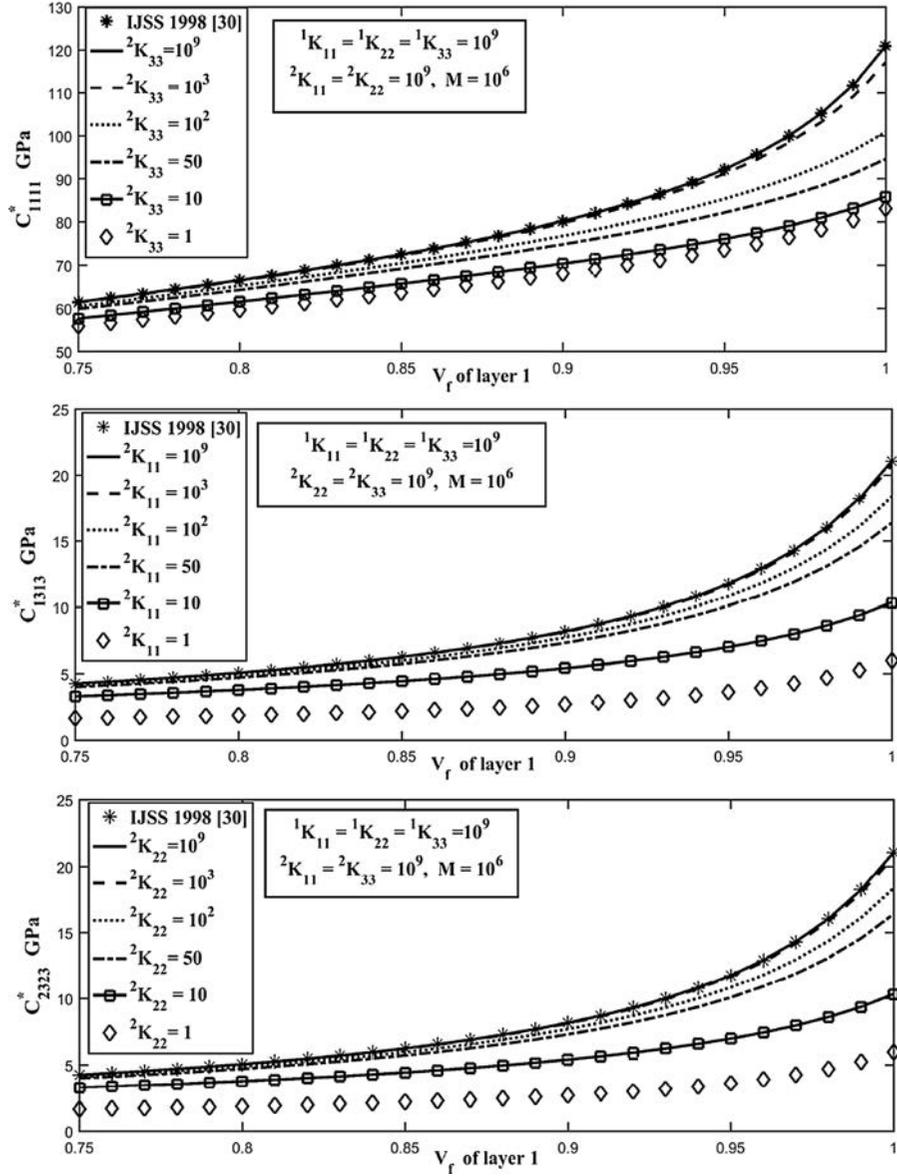
**Fig. 2** Effect of the imperfection parameter on the effective elastic coefficients  $C_{1111}^*$ ,  $C_{1313}^*$  and  $C_{2323}^*$  considering a bi-phase partition for the bi-laminate composite PZT-5A/Araldite
