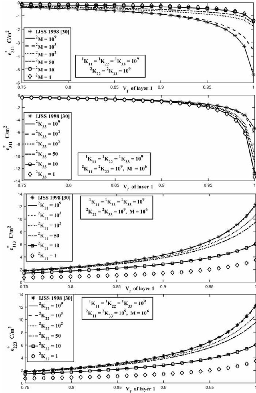
**Fig. 3** Effect of the mechanical/electrical imperfection parameters on the effective piezoelectric coefficients  $e_{311}^*$ ,  $e_{113}^*$  and  $e_{223}^*$  for a bilaminate composite PZT-5A/Araldite
