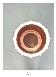
Fig. 2. (a) New probe built in this work, which has been installed right on the sample cell. The new probe is much more closer to the sample compared to the previous setup. (b) Front view of the RF shield. (c) Top view of the RF shield. In the modified setup the rungs of the coil were close to the sample and far away from the shield, and consequently the sensitivity has increased.
