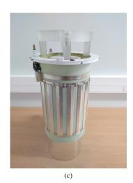
Fig. 1. (a) The device we used to hold the sample, and to apply a shear stress on the material (shear device). (b) Schematic view from the interior of the shear device inside the former bird-cage probe. In the former setup the probe was outside of the shear device, and as a result the rungs of the coil were far away from sample.
