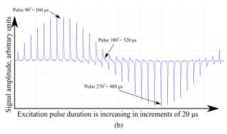
Fig. 5. Nutation curves of the new probe (a), and the previous probe (b). The length of the  $90^{\circ}$  pulse is  $60\mu$ s for the new probe compared to  $160\mu$ s for the previous probe. Although the noise level in (b) is much less than in (a) the setup in (a) in more sensitive for our experiment. In (b) we have more SNR simply because we have used a much larger sample. For a correct comparison the same sample has to be used for both probes.
