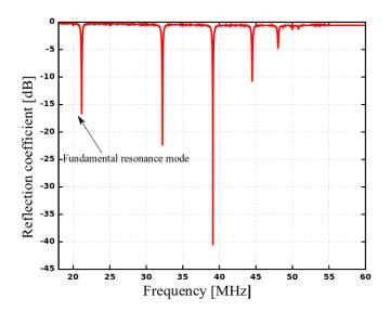
Fig. 4. Reflection coefficient,  $S_{11}$ , of the tuned and matched coil. As can be seen more than one resonances exist. For a low-pass bird-cage coil, the fundamental resonance corresponds to the lowest frequency. The resonance that occur at frequencies higher than 21.3 MHz do not produce a homogeneous  $B_1$  field.
