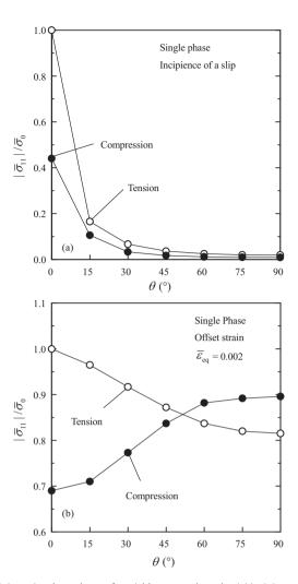
**Fig. 3.** Orientation dependence of re-yield stress evaluated at (a) incipience of a slip and (b) 0.2% accumulation of macroscopic equivalent plastic strain. Re-yield stress is normalized by one for  $\theta$  = 0° with uniaxial tension in subsequent loading stage, which is denoted by  $\tilde{\sigma}_0$ .
