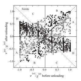
**Fig. 8.** Change of resolved shear stress,  $\tau^{(\alpha)}$ , before and after unloading for ferrite.  $\tau^{(\alpha)}$  is normalized by slip resistance,  $g^{(\alpha)}$ .
