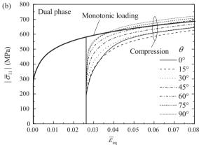
**Fig. 6.** Macroscopic stress–strain curve of dual-phase steel under uniaxial tension followed by (a) uniaxial tension and (b) uniaxial compression.
