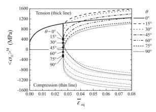
Fig. 11. Development of average tensile stress of martensite.
