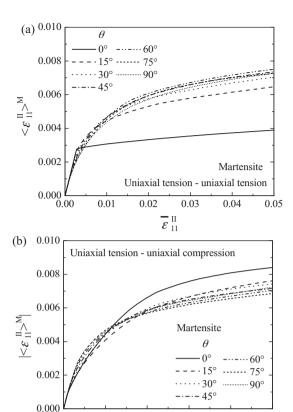
**Fig. 12.** Development of average strain for martensite as a function of macroscopic strain in subsequent loading stage.
