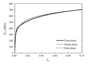
Fig. 1. Comparison of stress-strain curves predicted for single- and dual-phase steels with experimental result.
