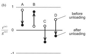
**Fig. 4.** Change of resolved shear stress,  $\tau^{(\alpha)}$ , before and after unloading stage. Resolved stress is normalized by corresponding slip resistance,  $g^{(\alpha)}$ . (a) Scatter diagram and (b) schematic illustration of change of  $\tau^{(\alpha)}$  in the first and fourth quadrants in (a).
