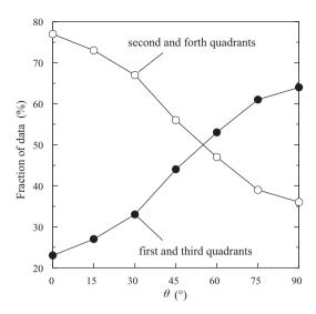
**Fig. 9.** Fraction of data belonging in the first and third quadrants and the second and forth quadrants in figure showing relationship between  $\Delta \tau^{(\alpha)}/\Delta \bar{\sigma}_{11}$  and  $\tau^{(\alpha)}/g^{(\alpha)}$  after unloading.
