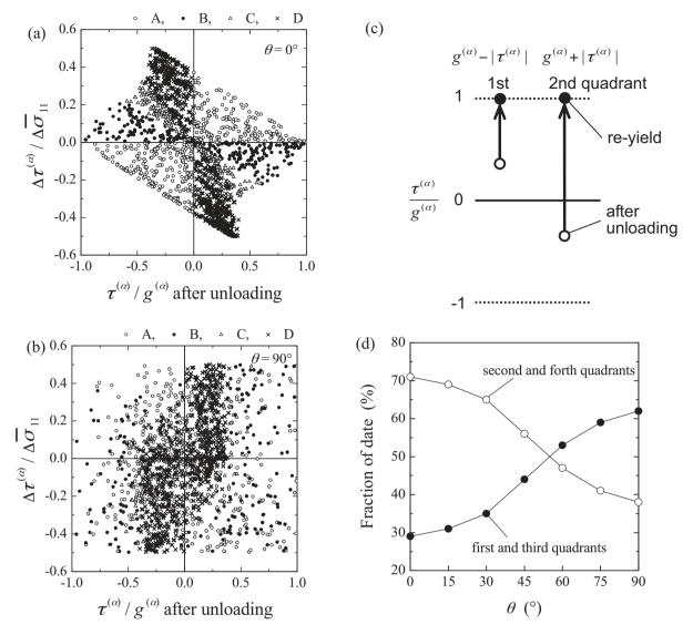
**Fig. 5.** Change of resolved shear stress due to uniaxial stress increment for (a)  $\theta = 0^{\circ}$  and (b)  $\theta = 90^{\circ}$  ( $\Delta \tau^{(\alpha)}/\Delta \bar{\sigma}_{11}$  corresponds to the Schmid factor for a slip system), (c) a distance of stress between unloaded state and re-yield state, and (d) fraction of data belonging to the first and third quadrants and the second and forth quadrants in (a), (b) and figures for other  $\theta$ .
