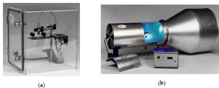
Figure 4. Standardized experimental setups for natural convection (a) and forced convection (b).
