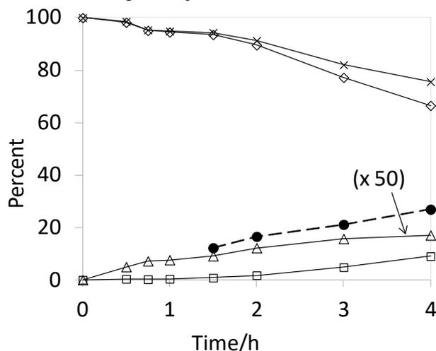
Figure 5- Time evolution of cyclooctene oxide yield (□), *trans*-cyclooctane-1,2-diol yield (Δ, x50), residual cyclooctene (◇), total (×), and cyclooctene oxide selectivity (● and dashed line) measured in the organic phase for the reaction of cyclooctene with H<sub>2</sub>O<sub>2</sub> (1.5 equiv) catalyzed by (BP)<sub>3</sub>[PMo<sub>12</sub>O<sub>40</sub>] (0.1%).
