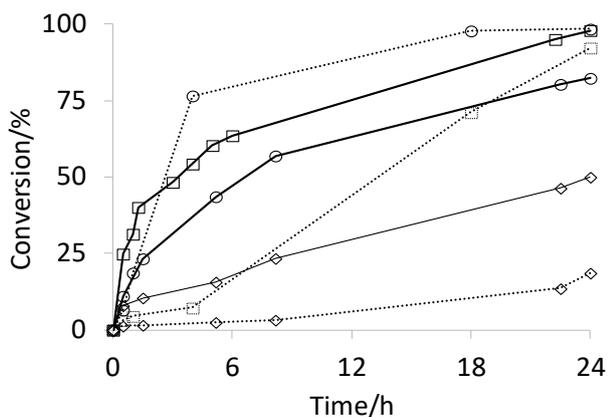
Figure 2 - Time dependence of the cyclooctene conversion in the presence of Q<sub>5</sub>[PMO<sub>12</sub>O<sub>40</sub>]. Q = BP (□) TBA (◇) CP (○). Oxidant = H<sub>2</sub>O<sub>2</sub> (dotted lines), TBHP (plain lines). Conditions: cyclooctene/oxidant/POM = 1000/1500/1. T= 80°C.
