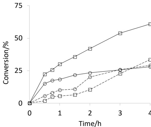
Figure 9- Cyclooctene conversion vs time for the cyclooctene epoxidation in presence of  $(BP)_3[PM_{12}O_{40}]$ . M = Mo (□), W (○); oxidant =  $H_2O_2$  (dotted lines) TBHP (plain lines). Conditions: cyclooctene/oxidant/POM = 1000/1500/1, T = 80°C.
