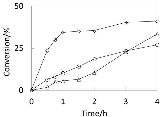
Figure 6- Cyclooctene conversion vs. time for the (BP)<sub>3</sub>[PMo<sub>12</sub>O<sub>40</sub>]-catalyzed epoxidation by aqueous H<sub>2</sub>O<sub>2</sub>. Conditions: (cyclooctene + additive)/H<sub>2</sub>O<sub>2</sub>/POM = 1000/1500/1. T= 80°C. Additive: none (Δ) (same as in Figure 2), cyclooctene oxide (○), *trans*-cyclooctane-1,2-diol (◇).
