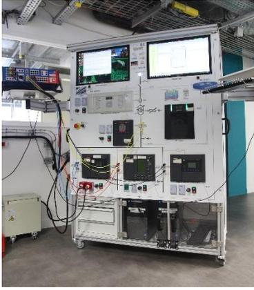
Fig. 4. Smart Grid Intelligent Substation coupled to a linear power amplifier
