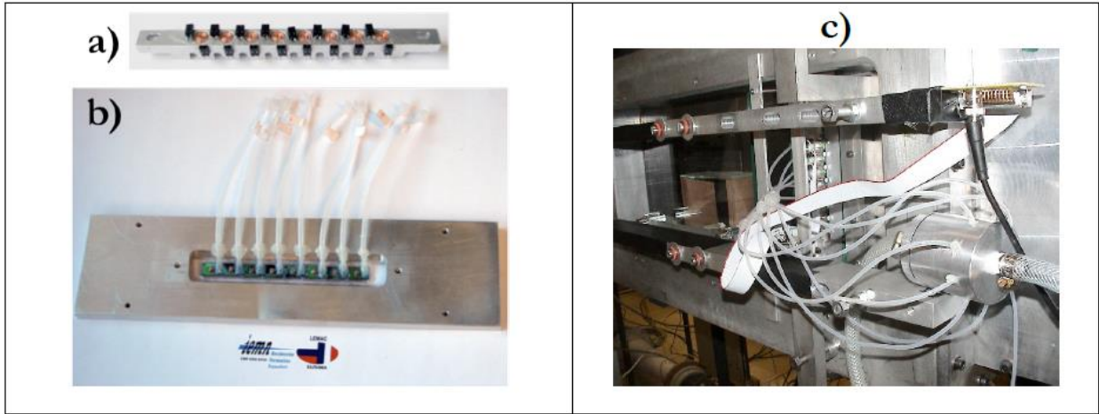
Figure 4: (a) Metallic bar supporting the coils; (b) Array of micro valves glued to the insert plate; (c) Photograph of the array integrated in the wind tunnel and view of the pressure distribution system.
