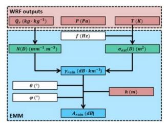
Fig. 2. Overview of rain attenuation computation using WRF outputs [6].
