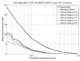
Fig. 6. Comparison of the rain attenuation CCDF for April 2017 in Kourou using different DSD models.
