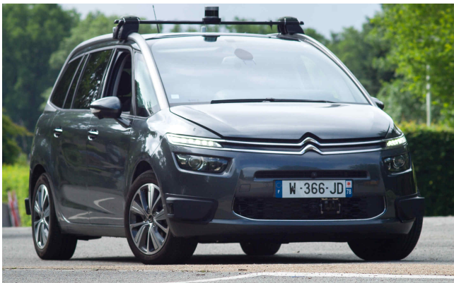
Fig. 10. Picture of the vehicle used in the real experiments. The car is equipped with a high-grade IMU, a LiDAR that outputs relative translation estimates, and a GPS-RTK used for ground-truth.
