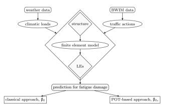
Fig. 1 General methodology, from monitoring to reliability
