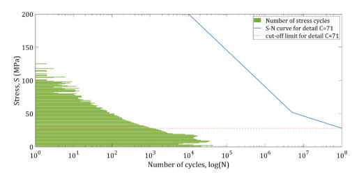
as  $S_D = 0.738 \times S_K = 52$  MPa, and the cut-off limit as  $S_L = 0.549 \times S_D = 28$  MPa. All stresses  $S < S_L$  do not contribute to the fatigue damage accumulation.
