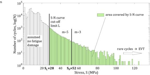
Fig. 8 Stress cycles histogram
