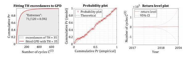
Fig. 11 Example of POT results for the range  $dS_2$ : (i) fitting GPD to histogram of  $C^{(2)}$ , (ii) probability plot, (iii) return level plot
