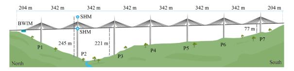
Fig. 4 Millau viaduct, position of SHM and BWIM systems
