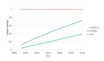
Fig. 12 Fatigue damage accumulation during the operational life of the viaduct, comparison of two methods
