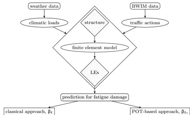
Fig. 1 General methodology, from monitoring to reliability
