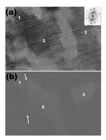
FIG. 6. (a) PV-HRTEM image of a thin (a few nanometers) (11–20) ZnO on R-sapphire. The inset is the Fourier transform. (b) Fourier filtered image of the image in Figure 4(a) using the  $(1-100)_{ZnO}$  spot. White arrows indicate BSFs.
