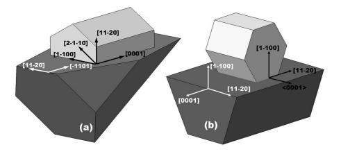
FIG. 1. Schematic representation of the epitaxial relationships between wurtzite nonpolar films with R-sapphire (a) and M-sapphire (b). The sapphire axes are in white and the GaN/ ZnO axes in black.
