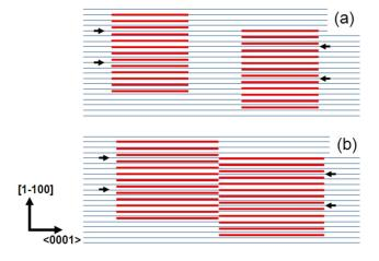
FIG. 8. (a) Schematic representation of the initial stage of the nucleation of (11–20) ZnO on R-sapphire. The sapphire (11–20) planes are represented in blue and the ZnO (1–100) planes in red. The black arrows indicate geometrical MDs. Two independent growth islands are shown. The crystalline directions of ZnO are indicated. (b) Coalescence of the two islands of Figure 8(a). The independent formation of geometrical MDs in the two islands result in a translation of the  $(1–100)_{ZnO}$  planes.
