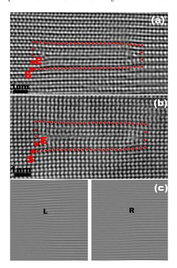
FIG. 3. (a) and (b) PV-HRTEM of BSF in a (11–20) oriented ZnO film. Burger circuits (from S to E) show that the BSF + PD groups correspond to a dissociated *c*-type dislocation (a) and an a+c-type dislocation (b). (c) PV-(0002) lattice images of the left (L) and right (R) edges of a BSF in a (11–20) oriented GaN film.
