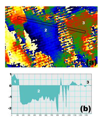
FIG. 7. (a) Phase image of the image in Figure 6(a) for  $(1-100)_{ZnO}$  planes. The phase reference is in region 3. (b) Profile of the phase in the rectangle drawn in Figure 7(a), the intensities being projected along the small side of the rectangle.
