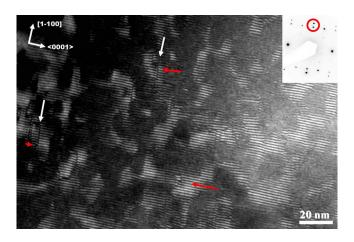
FIG. 5. PV- dark field image of a thin layer (a few nanometers) of (11-20) ZnO on R-sapphire. The inset is a selected area electron diffraction pattern where the  $(1-100)_{ZnO}$  and  $(11-20)_{sapphire}$  spots used for imaging are shown. White arrows indicate BSFs and red arrows edge dislocations. The ZnO axes are indicated.
