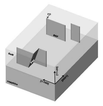
FIG. 2. Schematic representation of structural defects in an A-oriented wurtzite film on R-sapphire. The different kinds of defects are indicated. The wurtzite axes are also shown.
