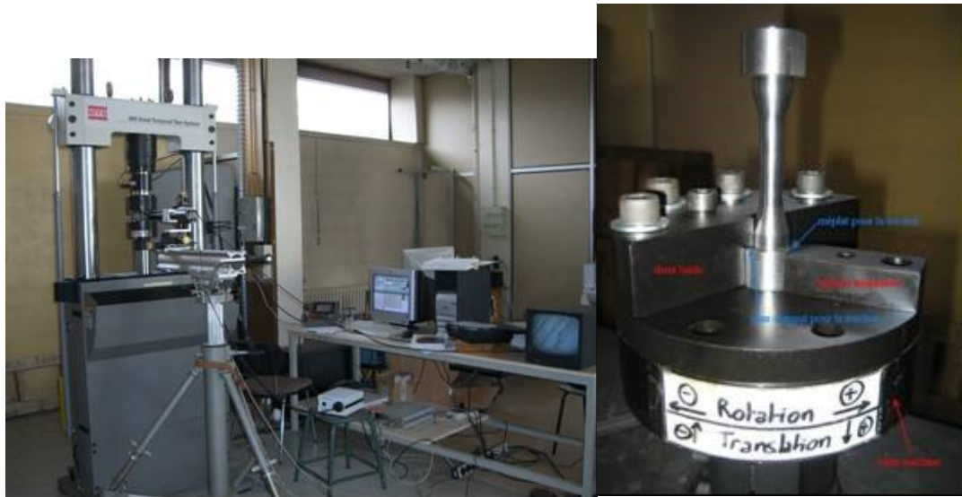
Figure 5: Fatigue Test Machine, Control Unit, and Test Specimen
