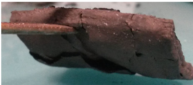
Figure 6 Example of char obtained after burning of algal/bentonite block (dimensions of the block after thermal degradation: 51 × 26 × 4.5 mm).
