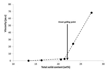
Fig. 6. Relation between PVOH/CAM (35/65) total solid content and viscosity.
