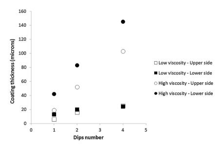
Fig. 9. Coating thickness versus dips number for EPS-HBCD coated with suspensions of low or high viscosity.
