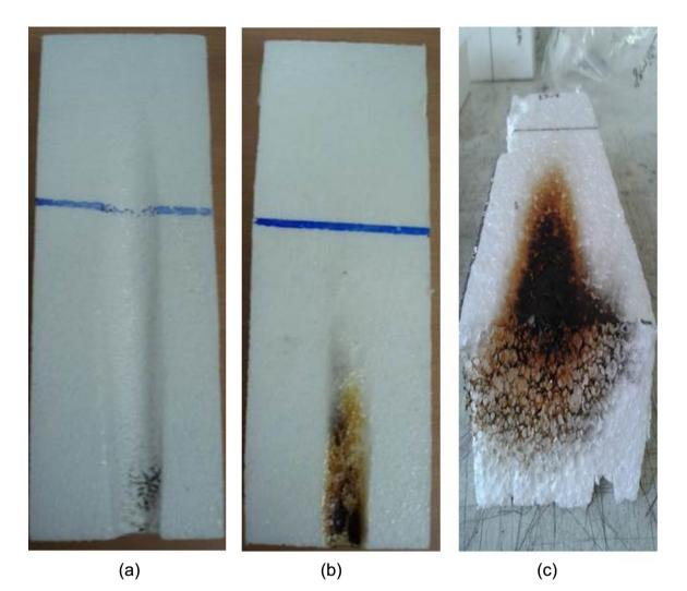
Fig. 20. Residue of non-coated EPS-HBCD (a), EPS without HBCD coated with CAM/PVOH 65/35 (b) and after the removal of its surface layer on the lower side (c).
