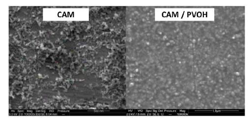
Fig. 3. SEM images of filler CAM (scale bar 500 nm) and dried film microstructure (scale bar 1 µm).
