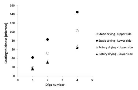
Fig. 12. Coating thickness versus dips number for EPS-HBCD coated with suspension of high viscosity and dried using static or rotary drying.
