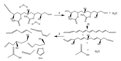
Scheme 1. Pyrolytic degradation steps of poly(vinyl alcohol) (PVOH) [31].
