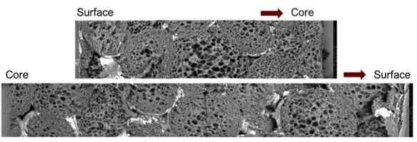
Fig. 15. The CAM/PVOH penetration into the core of EPS without HBCD for one dip during 18 h.
