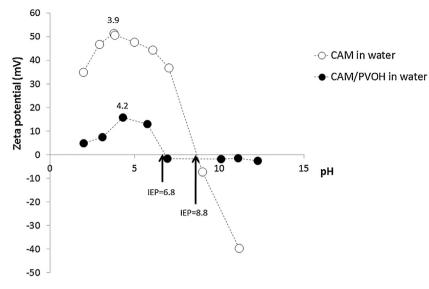
Fig. 5. Influence of pH on the zeta potential of aqueous suspension of CAM and CAM/PVOH.
