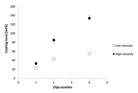
Fig. 8. Coating level versus dips number for EPS-HBCD coated with suspensions of low or high viscosity.
