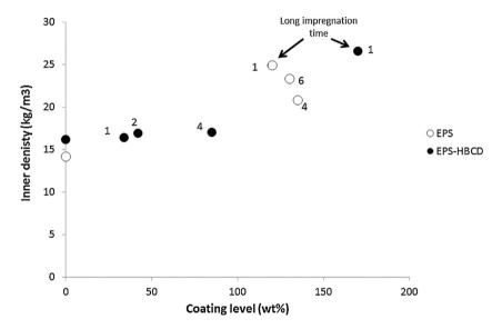
Fig. 18. The density evolution versus the coating level for various coated EPS foams (labels correspond to the dips number).
