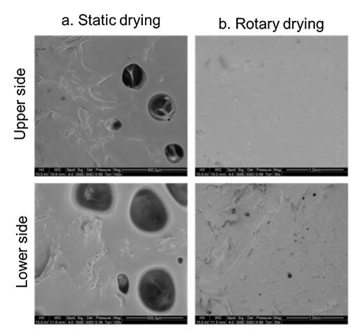
Fig. 13. Influence of drying method on coating surface texture (scale bars: 400 µm-top and left, 500 µm-bottom and left, 1 mm-right).
