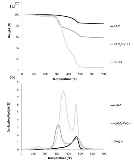
Fig. 7. Weight (a) and derivative weight (b) curves versus temperature under N<sub>2</sub> at heating rate of 10 °C/min for CAM boehmite, PVOH and CAM/PVOH 65/35.
