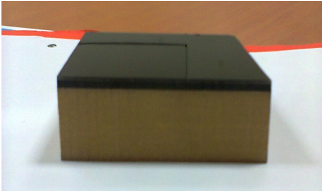
Fig. 2. Coated wood two-layer composite (coating has already been partially decomposed on the picture).
