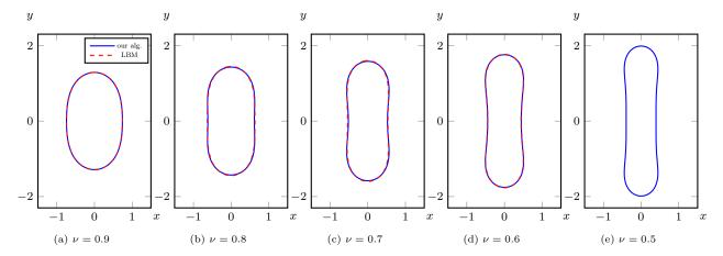
Figure 8: Comparison of the 2D equilibrium shapes obtained by alg. 6 with the ones obtained by [26] using a lattice-Boltzmann method for reduced volumes  $\nu = 0.9, 0.8, 0.7$  and 0.6. We also give our result for a reduced volume  $\nu = 0.5$ .
