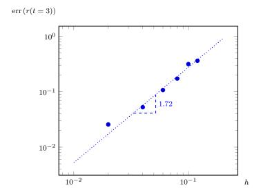
Figure 4: Evolution of the error  $\operatorname{err}(r(t=3)) \equiv |r_h(t=3) - r(t=3)|$  of the radius of the circle at t=3 as a function of the mesh size. The figure also shows the best mean-square fit of the data by a power function  $14.48\,h^{1.72}$ . Note however that the displayed slope is not strictly equivalent to the usual convergence order, as discussed above.
