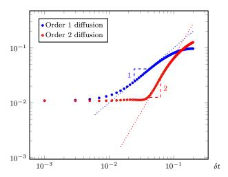
Figure 1:  $L^2$  error on curvature estimates using the Order 1 eq. (36) and Order 2 eq. (37) diffusion methods as a function of the diffusion time-step  $\delta t$ . We observe the expected convergence orders as the time-step decreases, and a saturation of the error for low time-steps which is related to space discretisation error terms.
