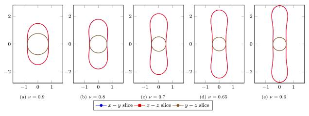
Figure 16: Cut slices in the x-y, x-z and y-z planes of the 3D prolate vesicles equilibrium shapes displayed in fig. 11. These cuts highlight the good symmetry preserving property of our algorithm despite the absence of any symmetry enforcing method.
