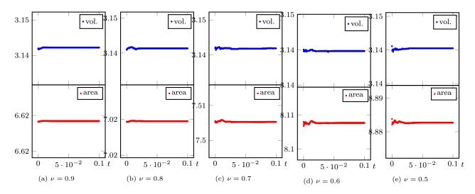
Figure 9: Evolution of the 2D vesicle volume and "area" (perimeter in this case) with the volume- and area-preserving alg. 6. The algorithm displays very good conservation properties: the relative volume and area changes are less than respectively  $1 \cdot 10^{-4}$  and  $5 \cdot 10^{-4}$  for the most difficult  $\nu = 0.5$  case, and the final equilibrium shapes volumes and areas relative changes are  $\lesssim 1 \cdot 10^{-5}$  for all the cases.
