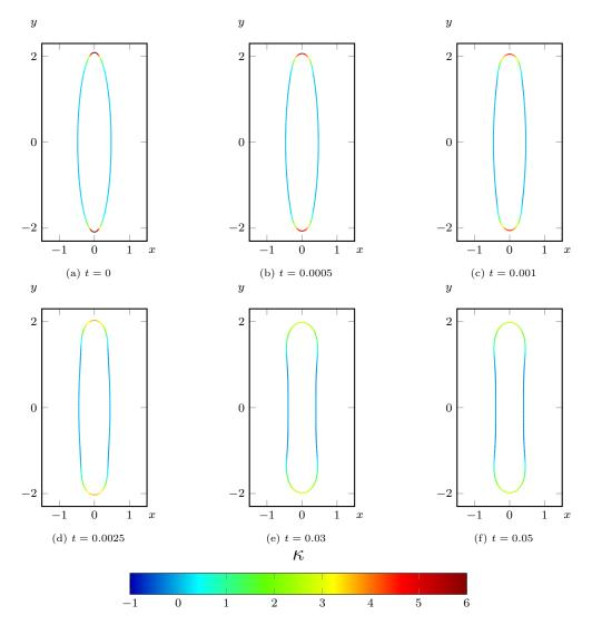
Figure 7: Convergence of alg. 6 to an equilibrium shape for the  $\nu=0.5$  case, starting from an ellipse with semi-major and -minor axes 2.09021 and 0.478421. The curves are colored with the value of the curvature.
