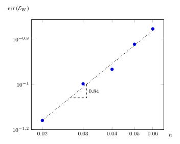
Figure 20: Relative error of the Willmore energy of our three-dimensional vesicle equilibrium shape for the  $\nu=0.65$  case as a function of the mesh size. The error is computed as  $\left(\mathcal{E}_W-\mathcal{E}_W^{th}\right)/\mathcal{E}_W^{th}$  with  $\mathcal{E}_W^{th}$  taken from [52], and the mesh sizes range from  $h\approx0.02$  to  $h\approx0.06$ . The plot is in log-log scale.
