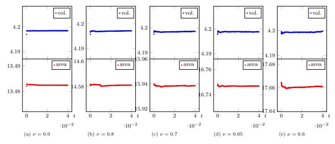
Figure 13: Evolution of the 3D oblate vesicle volume and area with the volume- and area-preserving alg. 7. The 3D algorithm also displays good conservation properties: the relative volume and area changes are respectively  $\lesssim 5 \cdot 10^{-5}$  and  $\lesssim 2 \cdot 10^{-4}$  for all the cases.
