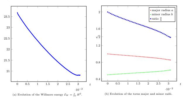
Figure 6: Willmore energy and geometrical quantities of the torus. We observe that the flow decreases the energy to about 20.8, which is within 5% from the theoretical Clifford torus energy  $2\pi^2 \approx 19.74$ . We also observe that at equilibrium, the ratio between the radii is indeed about  $\sqrt{2}$ . Beyond t=3, the surface leaves the toroidal class, and the computed a and b are not anymore relevant (see above).
