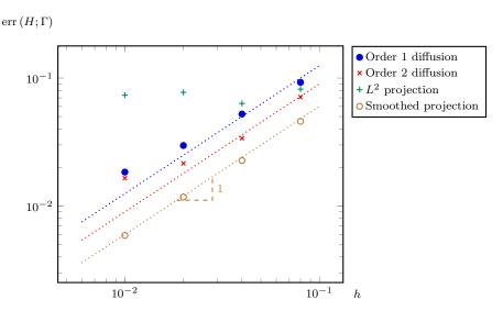
Figure 2: Evolution of the  $L^2$  error as a function of the mesh size for the different methods. The  $L^2$  projection shows no evident convergence while the Order 1 diffusion, the Order 2 diffusion and the Smoothed projection methods yield linear convergence.
