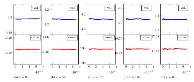
Figure 17: Evolution of the 3D prolate vesicle volume and area with the volume- and area-preserving alg. 7. The 3D algorithm also displays good conservation properties: the relative volume and area changes are respectively  $\lesssim 5 \cdot 10^{-6}$  and  $\lesssim 3 \cdot 10^{-5}$  for all the cases.
