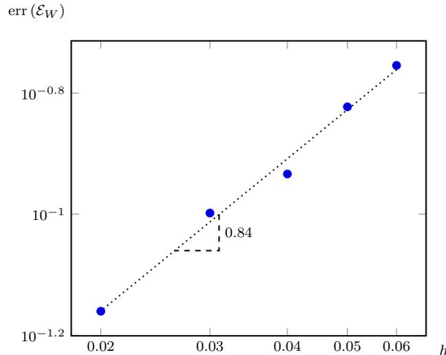
Fig 20: Relative error of the Willmore energy of our three-dimensional vesicle equilibrium shape for the  $\nu = 0.65$  case as a function of the mesh size. The error is computed as  $(\mathcal{E}_W - \mathcal{E}_W^{th}) / \mathcal{E}_W^{th}$  with  $\mathcal{E}_W^{th}$  taken from [52], and the mesh sizes range from  $h \approx 0.02$  to  $h \approx 0.06$ . The plot is in log-log scale.
