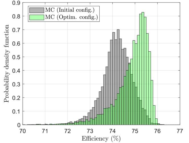
Fig. 9. PDF of the efficiency of the wireless power transfer improved (green) by increasing the nominal values of the input variables  $L_2$ ,  $C_4$ ,  $slot_{\{x,y\},RX}$ ,  $C_3$ ,  $g_{\{x,y\},RX}$  by  $2\sigma$ , where  $\sigma$  is given Table I, according to the circle of correlation given in Fig. 8.
