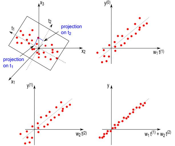
Fig. 1. Top left represents the construction of two principal components in the initial  $\mathbf{X}$  space. Top right and Bottom left illustrate the prediction of  $y^{(0)}$  and  $y^{(1)}$ , respectively. Bottom right shows the final prediction of the output  $y$ .
