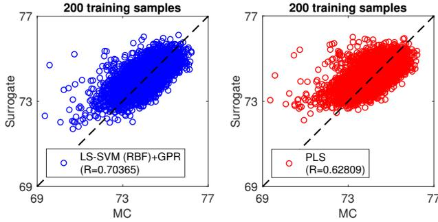
Fig. 3. Scatter plot of the WPT efficiency computed by the PLS surrogate model (red circles), the mean value of the LS-SVM (RBF)+GPR surrogate model (blue circles) vs. the actual numerical model with 10,000 MC realizations. The dashed line illustrates the perfect agreement between the models.
