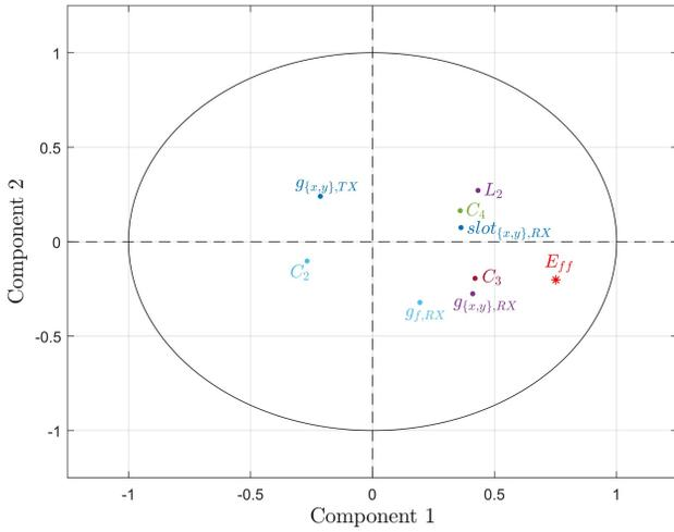
Fig. 8. Circle of correlation representing the projection of the input variables and the output variable (WPT efficiency  $E_{ff}$ ) onto the plane defined by the first two PLS components. It shows a strong positive correlation between the input variables  $L_2$ ,  $C_4$ ,  $slot_{\{x,y\},RX}$ ,  $C_3$ ,  $g_{\{x,y\},RX}$  and the output variable  $E_{ff}$  since their projections are in the same direction and at a significant distance from the origin.
