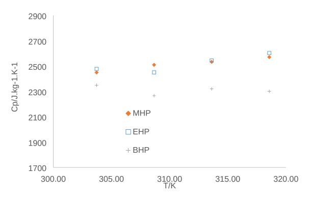
Fig. 9. Variation of specific heat capacity of intermediates versus temperature.
