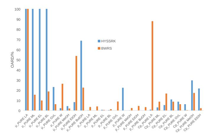
Fig. 10. Experimental and simulation comparison for pure solution: viscosity, density and specific heat capacity.
