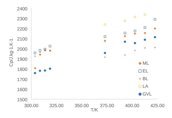
Fig. 5. Evolution of specific heat capacity of the pure compounds with temperature.
