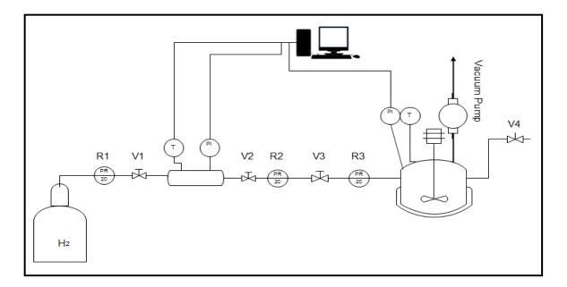
Fig. 1. Reactor setup for the production of intermediaries.
