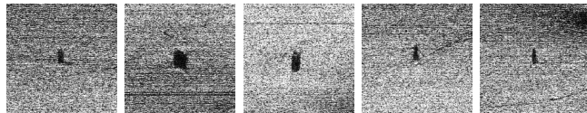
Fig. 1. Different underwater rocks perceived with one side-scan sonar. These observations are view-point dependent and the sonar images are noisy, which makes it difficult to distinguish one rock from another only from image processing. The sonar images of this paper have been collected by the Daurade robot (DGA-TN, Shom, Brest) equipped with a Klein 5000 lateral sonar.
