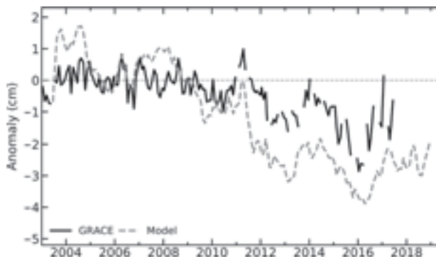
FIG. 2.28. Global average terrestrial water storage anomalies from GRACE (black) and from a GRACE data assimilating land surface model (gray), in cm equivalent height of water relative to a 2005–10 mean baseline.
