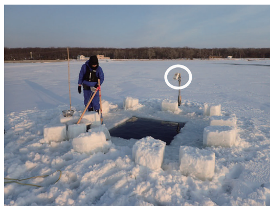
Fig. 14. Photographs of pool experiments for the whole site to examine the effects of snow on the sea ice structure at the early growth stage (a), where a white circle denotes a monitoring camera, and ice sampling (b).
