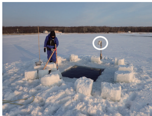
Fig. 14. Photographs of pool experiments for the whole site to examine the effects of snow on the sea ice structure at the early growth stage (a), where a white circle denotes a monitoring camera, and ice sampling (b).
