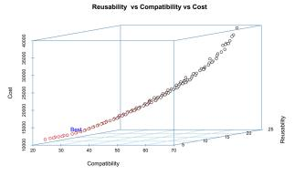
Fig. 12 Pareto Front obtained by the NSGA II Mixte Continu-Entier-Booléen LBCE algorithm
