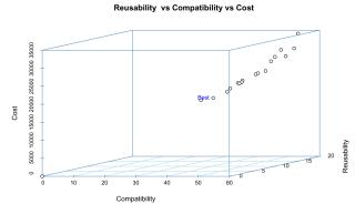
Fig. 13 Pareto Front obtained by the MIB MOGA Continu-Entier-Booléen (LBCE) algorithm
