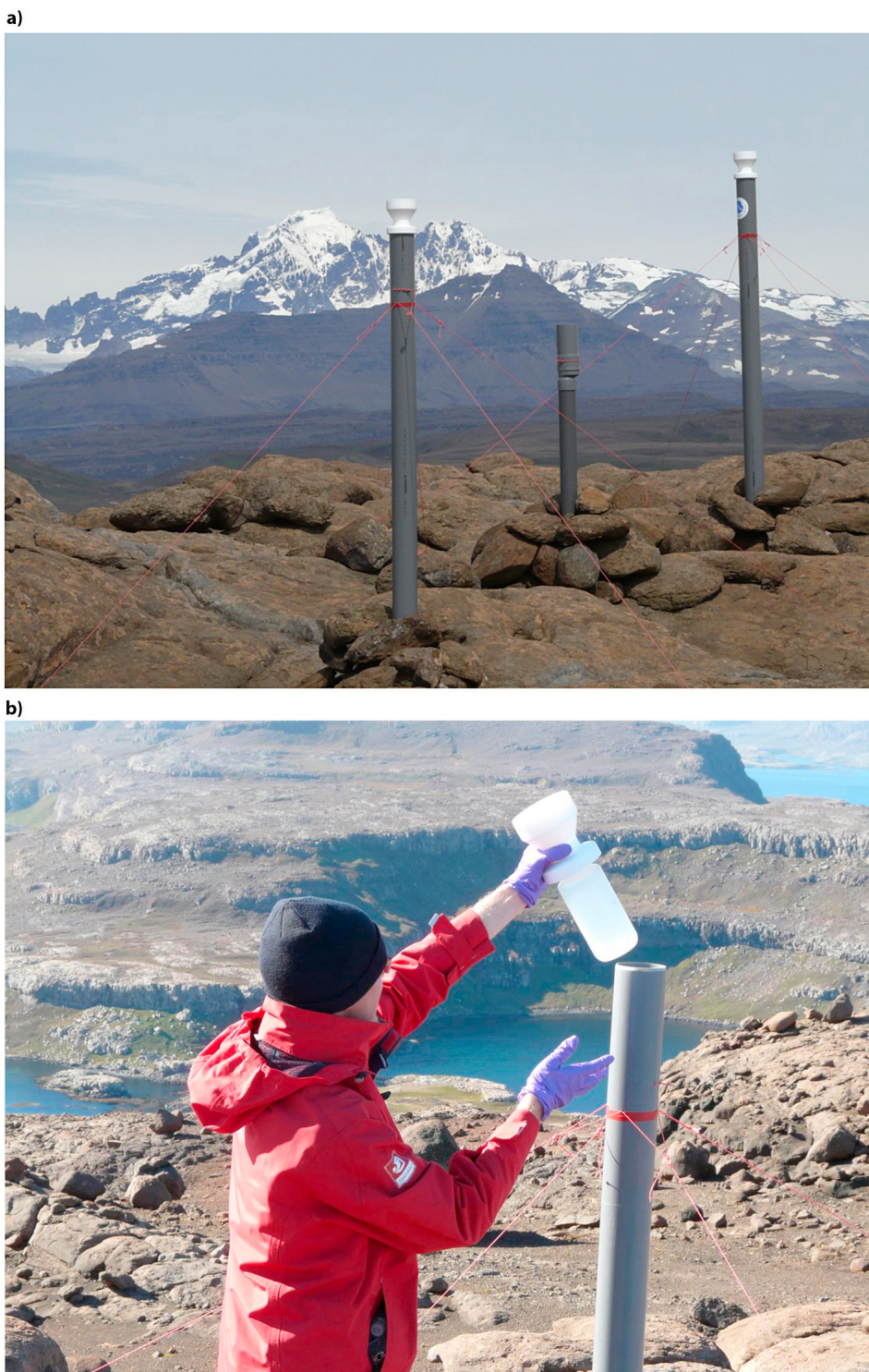
Figure 2. (a) Deposition collectors with duplicate sampling and bottle holder pipes; (b) detail of the deposition device.
