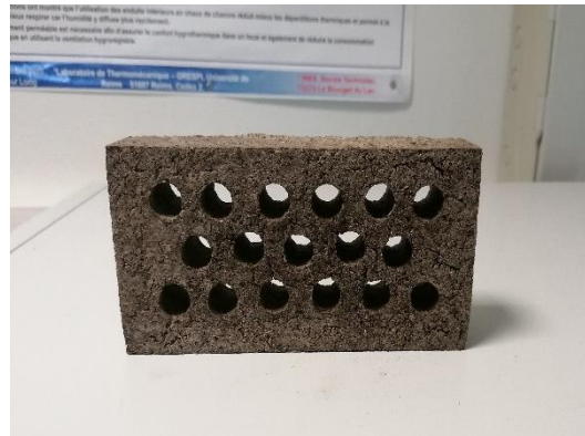
Figure 15 : Brick sample dried with lyophilizer
