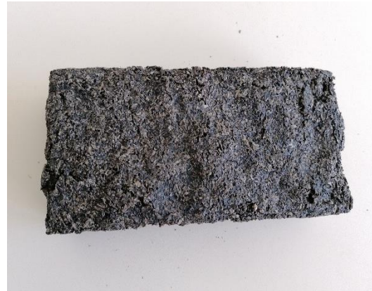
Figure 14 : Brick sample dried with the ventilated oven
