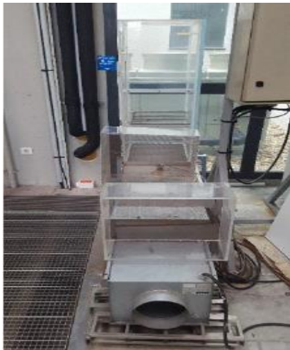
Figure 10 : Hot air drying tower
