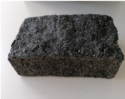
Figure 14 : Brick sample dried with the ventilated oven
