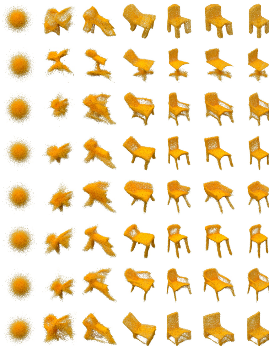
Fig. 16: Generating flow for sampled point clouds from the Chair model.
