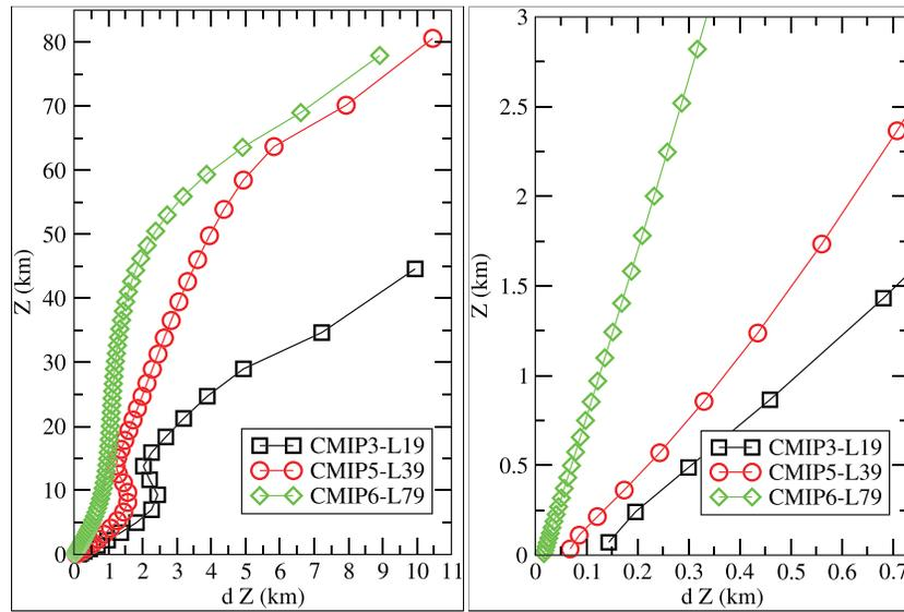
**Figure 1.** LMDZ vertical grids used for the reference configurations of the successive phases of the CMIP exercise with the IPSL model showing the altitude in y axis as a function of the layer thickness in x. A focus on the first 3 km is shown in the right panel.
