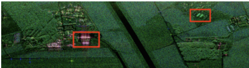
Figure 4. PolSAR image of the former Air Force Base of Bretigny acquired by ONERA (RAMSES, X-band) in the Pauli basis. The sensor trajectory is parallel to the top of the figure. Red rectangles refer to selected areas.
