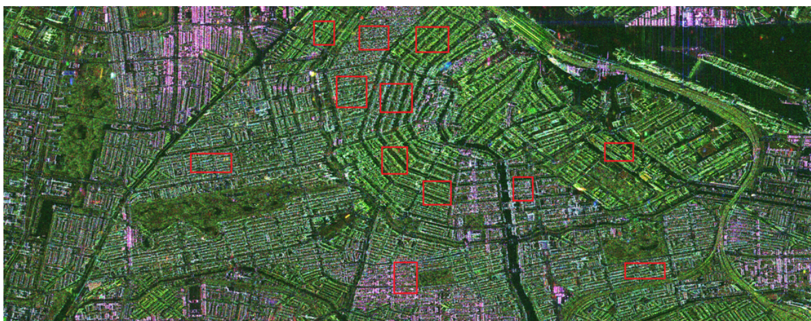
Figure 8. PolSAR image of Amsterdam acquired by TerraSAR-X (X-band) in the Pauli basis. The sensor trajectory is parallel to the left side of the figure. Red rectangles refer to selected areas.
