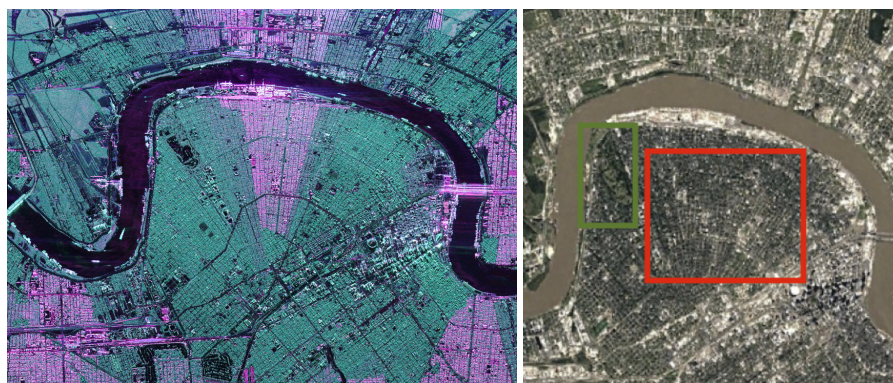
Figure 2. New Orleans, Louisiana, U.S. (Left) PolSAR image acquired by UAVSAR in the Pauli basis (double-bounce in red, single scattering in blue, cross-polarization in green). The sensor trajectory is parallel to the top of the figure; (right) Google Earth image of the same region acquired by Landsat and Copernicus.
