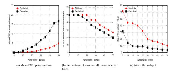
Fig. 5. Performance Study between centralized and blockchain-supported decentralized achitectures
